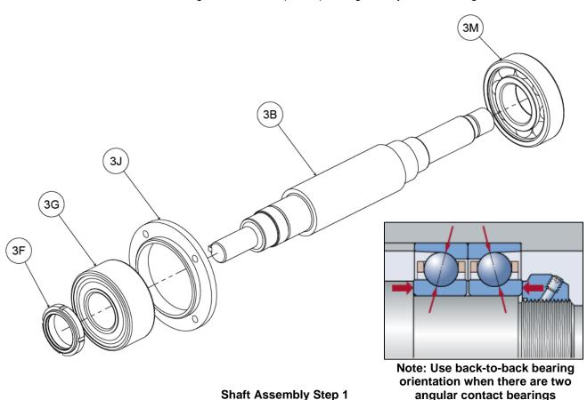
1. Install the outboard bearing retaining cover (3J/--), outboard bearing (3G/62B) and locknut (3F/62C) onto the shaft (3B/62). Then install inboard bearing (3M/62A) onto shaft. It is recommended that a bearing heater be used when installing bearings to avoid damage to the races. Be sure the bearing seats against the shoulder of the shaft. If the pump is grease lubricated, hand pack the bearings with the appropriate grease (reference lubrication) after they are seated on the shaft.
