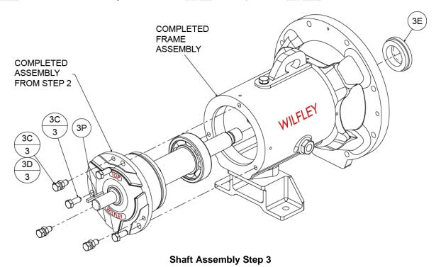
3. Install the inboard oil seal (3E/76) into the inboard bearing cover (2E/61J). To avoid damage, lubricate the oring (3H/72A) with light oil and slide the assembly into the frame (2A/61). The word "top" on the carrier (3A/72) must face up. Attach the bearing carrier with three retaining bolts (3C/75), jacking bolts (3C/75) and jam nuts (3D/72B). Attach square key (3P/62D) onto shaft (3B/62).
