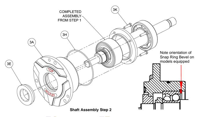
2. Install the outboard oil seal (3E/76) into the bearing carrier (3A/72). Be sure that the notch/opening faces down to allow for oil drainage. Install o-ring (3H/72A) onto bearing carrier. Slide bearing carrier over outboard bearing (3G/62B) and attach rear bearing retainer cover (3J/74) with cap screws (3K/74A).
