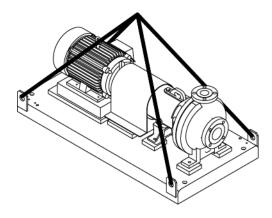
**Complete Pump Assembly Lifting**
